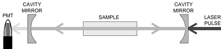
**FIGURE 3. Schematic of cavity ringdown spectroscopy (CRDS) apparatus.**
