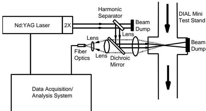
FIGURE 16. LIBS experimental setup.
