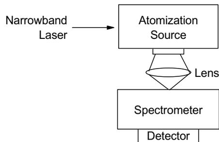
**FIGURE 10. Schematic of the laser induced fluorescence spectrometry technique.**
