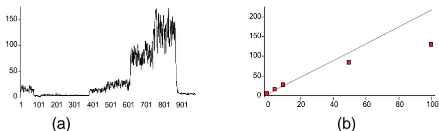
**FIGURE 4. (a) Time scan monitoring data for chromium (Cr (I) 359.35 nm), with metals introduced into the stack, water introduced into the stack, and Cr calibration spikes added to the sampled gas stream. (b) Calibration curve for Cr, generated from the time scan data.**
