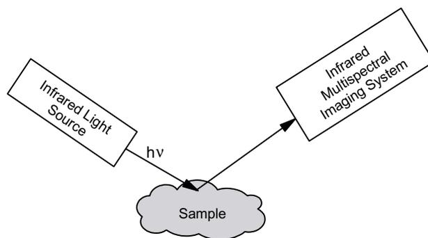
**FIGURE 12. Schematic of infrared diffuse reflectance multispectral imaging technique (final configuration).**
