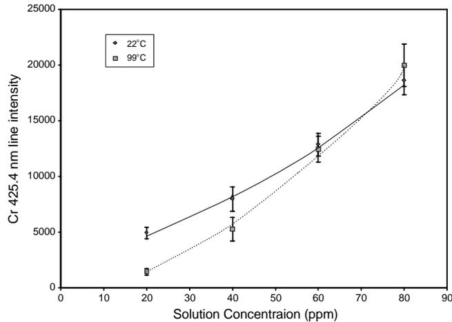
**FIGURE 18. Cr calibration data at different gas temperatures.**
