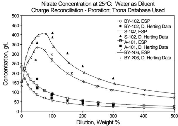
**FIGURE 13. Comparison of the ESP predictions of nitrate concentration with experimental data of Herting.<sup>7,8</sup>**
