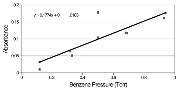
**FIGURE 8. Absorbance measurements for benzene in 730 Torr of nitrogen with diode laser temperature set at 35°C.**
