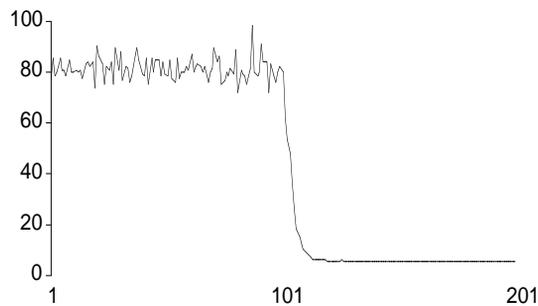
**FIGURE 3. Time scan emission monitoring for beryllium (Be (II) 313.04 nm), obtained for the introduction of a 100-ppm Be solution and a water blank, using the ultrasonic nebulizer (stack not connected).**
