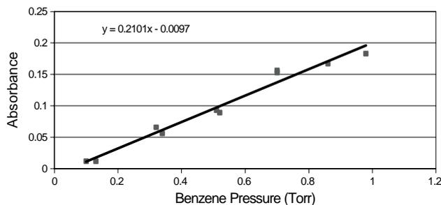
**FIGURE 9. Absorbance measurements for benzene in 730 Torr of air with diode laser temperature set at 35°C.**
