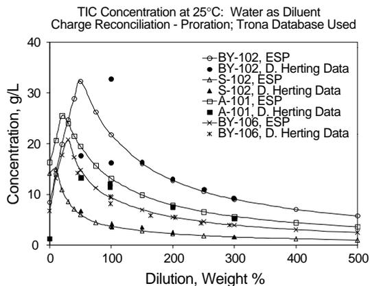
**FIGURE 15. Comparison of ESP predictions of TIC concentration with experimental data of Herting.<sup>7,8</sup>**
