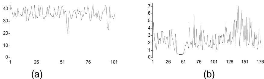
**FIGURE 6. Time scan monitoring for (a) chromium (Cr (I) 359.35 nm) and (b) beryllium (Be (II) 313.11 nm) during the second RM-29 sampling conducted on September 16. The detector integration time used was 3-s per point.**
