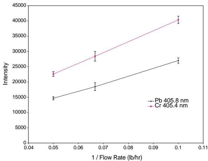
FIGURE 17. Atomic line intensity at different gas flow rates.
