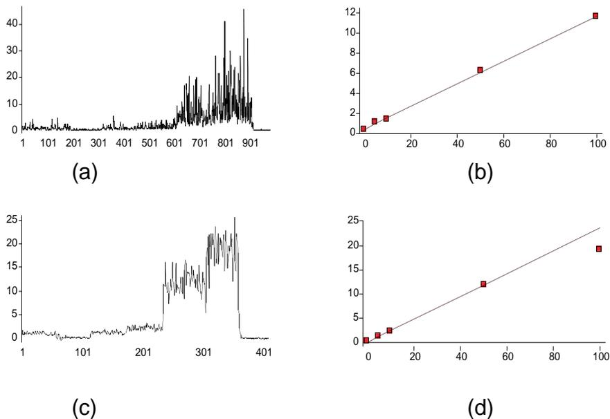
**FIGURE 5.** Time scan calibration spiking data for (a) beryllium (Be (II) 313.11 nm) and (c) lead (Pb (I) 405.78 nm), with metals introduced into the stack, water introduced into the stack, and calibration spikes added to the sampled gas stream. Calibration curves for (b) Be and (d) Pb, generated from the time scan data.
