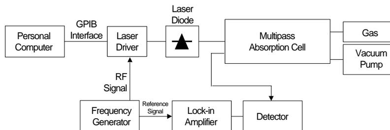
**FIGURE 7. Experimental configuration for diode laser absorption spectrometry**
