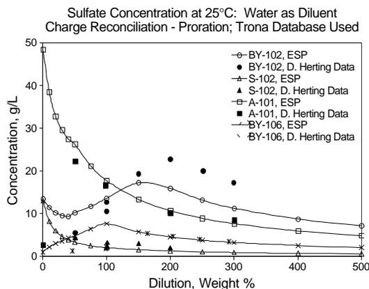
**FIGURE 14. Comparison of ESP predictions of sulfate concentration with experimental data of Herting.<sup>7,8</sup>**
