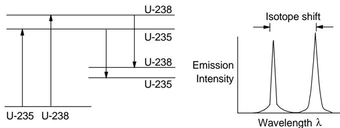
**FIGURE 11. Schematic of isotopic energy shifts and the associated LIF spectrum.**
