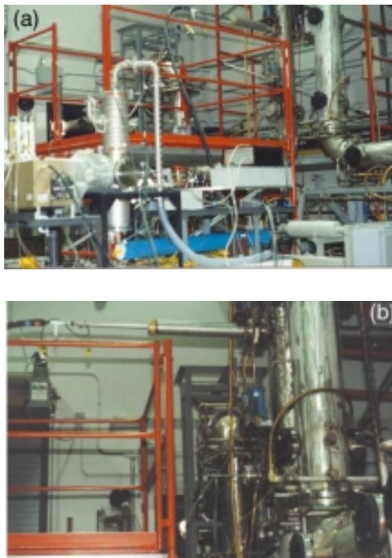
**FIGURE 2. (a) The continuous sampling air-ICP system connected to the combustion test stand at DIAL. Near the top of the photograph, the glass lined sampling probe is shown inserted into a vertical section of the test stand and connected to the black heat traced sample line. (b) The air-ICP sampling probe, inserted into the stack, showing the nebulizer spike location – the white Teflon tee between the probe and the sample line.**
