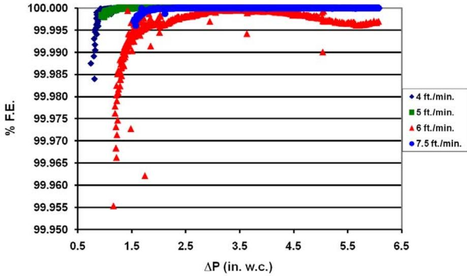
Figure 6. Trends in Initial Filter Efficiency as a Function of Media Velocity.
