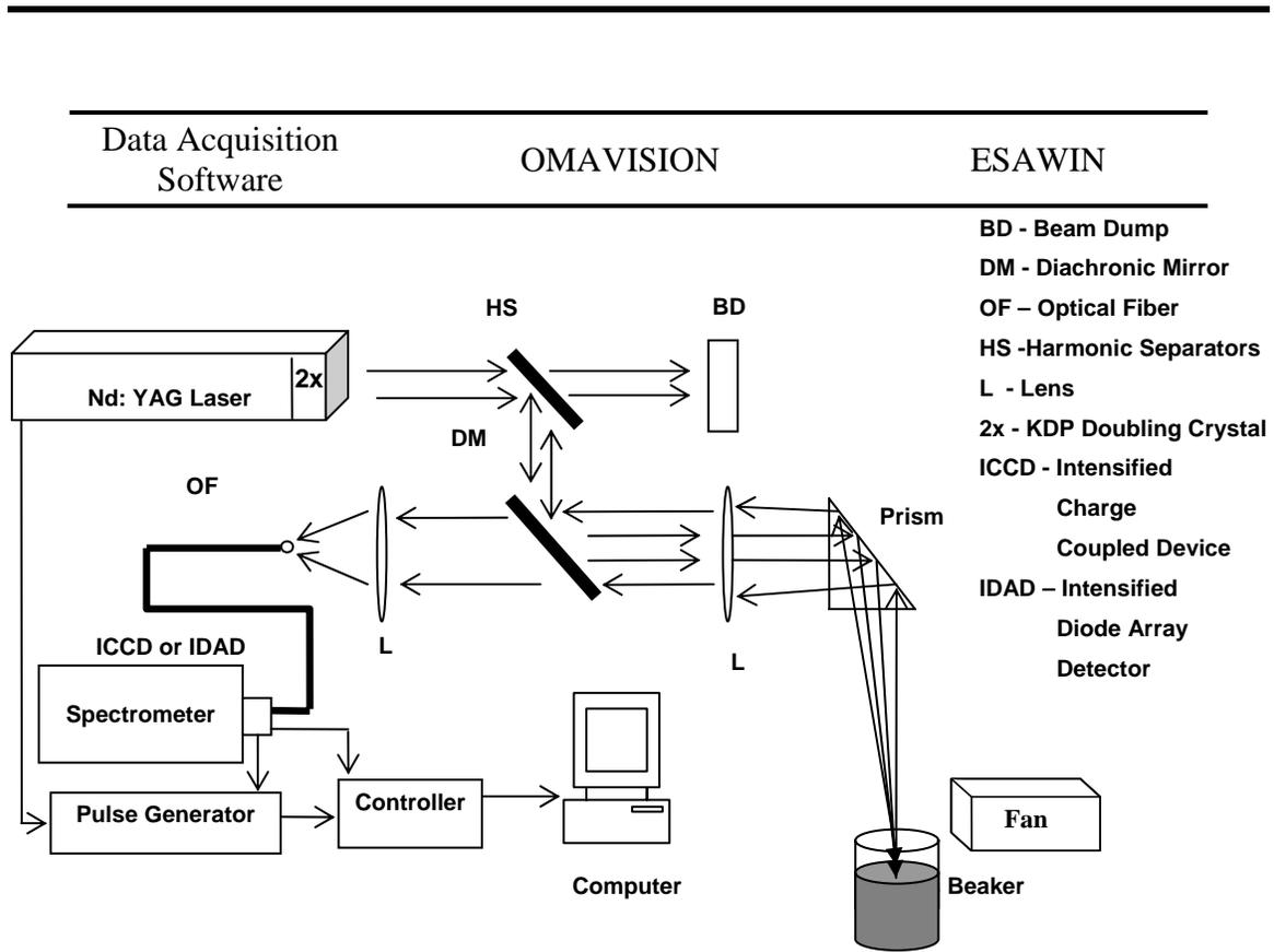
Figure 4 Schematic diagram of LIBS measurement apparatus.
