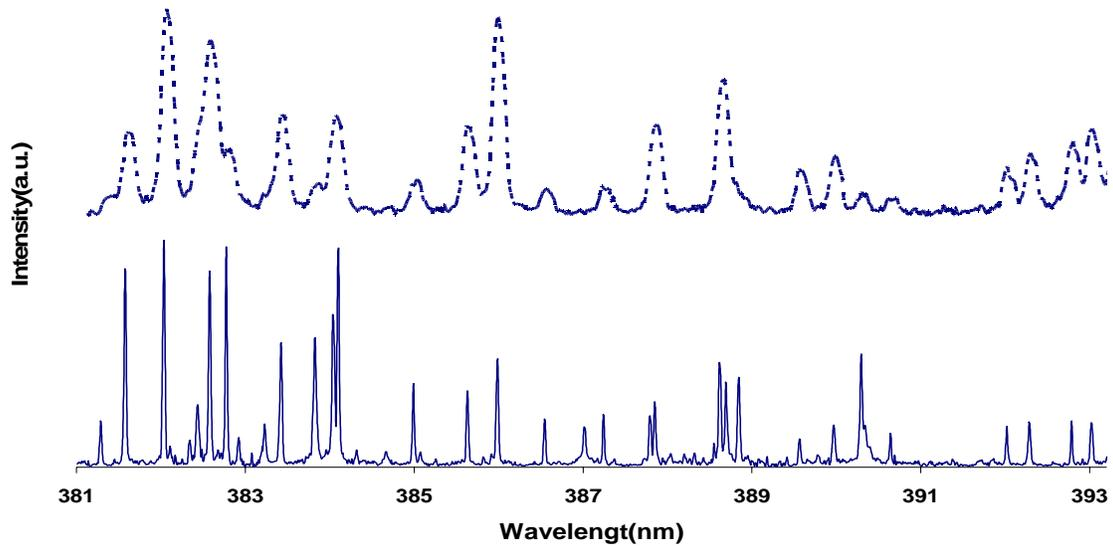
Figure 5 LIBS spectra of Sludge Receipt and Adjustment Tank slurry around 386 nm. The spectra of dashed line and solid line are recorded by Czerny-Tuner and Echelle spectrometers, respectively.
