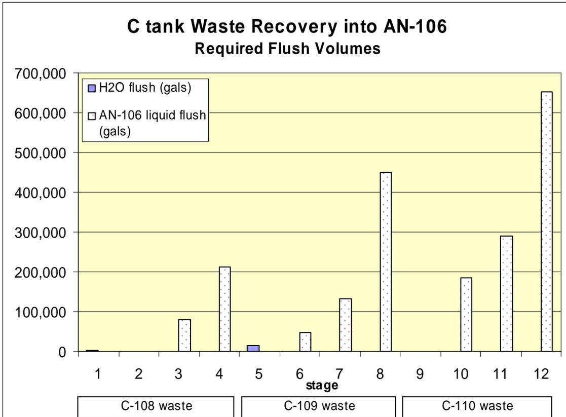
**Figure 9 Flush Volumes for C tank Recovery into AN-106**
