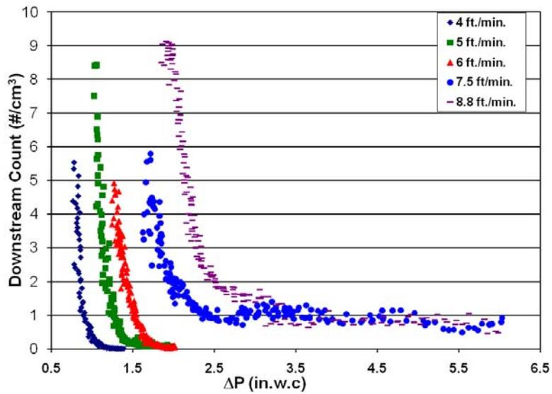
Figure 7. Trends in Downstream Particle Count as a Function of Media Velocity.
