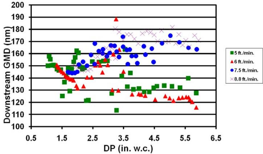
Figure 8. Trends in Downstream Count Median Diameter as a Function of Media Velocity.
