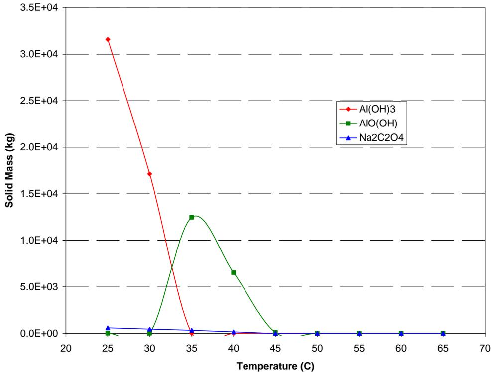
Figure-3 Effect of temperature on Batch 5 sludge with 140 kgal of 50% caustic added.
