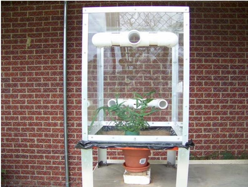
**Figure 18. Setup of the sunlit chamber study on mercury uptake by fern. Fern was planted in a pot containing clean soil under the chamber.**
