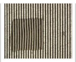
DIAL has developed a sensitive technique for measuring small variations in surface topography. The technique – called Fourier transform profilometry – is capable of detecting variations of a tenth of a millimeter on the surface of large objects such as walls. The U.S. Army has recently begun using this technique to quantify in real-time the patterns arising from explosions from experimental munitions. The technique can also be an extraordinarily useful non-contact quality control tool.
