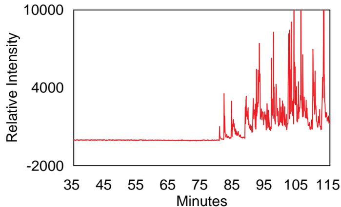
**Figure 3. The variation in the intensity of the 520.9-nm Ag I spectral line with time.**
