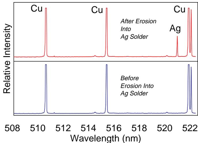
**Figure 2. The emission spectra in the 510 to 522-nm region before (bottom) and after (top) the electrode has eroded into the doped region of the back electrode of the dc arc.**
