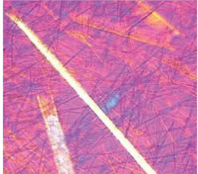
Figure 2. Polarized light microscope image of sodium phosphate dodecahydrate crystals.
