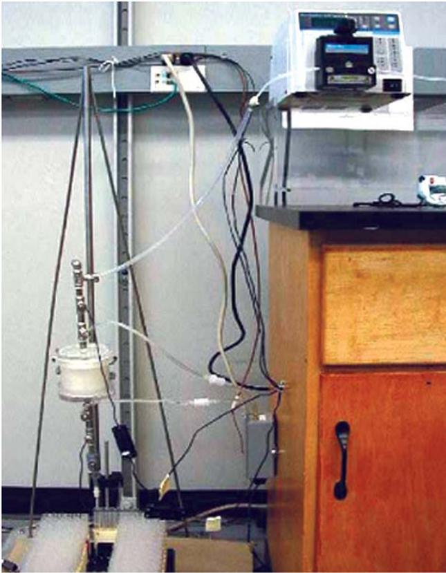
Figure 1. The flow through configuration of the SDFM consists of an acrylic column, a peristaltic pump for diluent addition, and a fraction collector.
