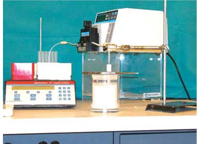
Figure 2. All operations in the DASR configuration of the SDFM are performed through a salt well.
