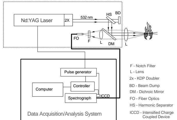
Fig. 2. Raman probe schematic.
