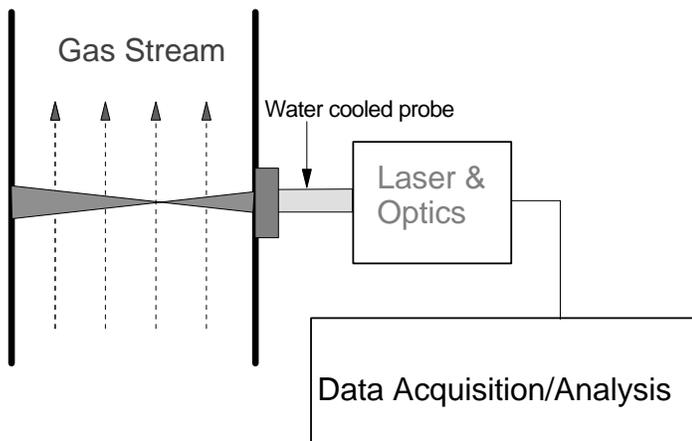
*Fig. 3. Raman probe setup in a furnace.*
