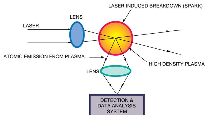
**Figure 1. Principle of laser-induced breakdown spectroscopy.**
