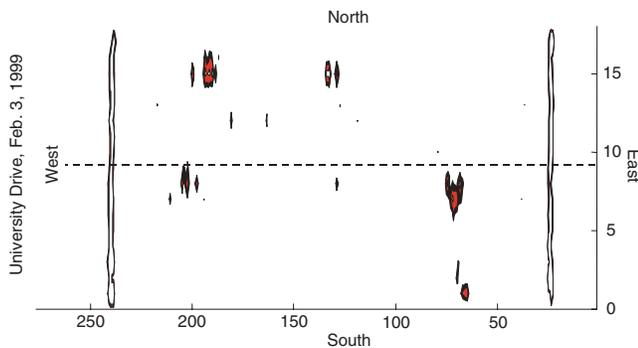
*Figure 3. Data collected from the University Drive Bridge over Highway 12, Starkville, MS. The dark bands on either end represent the expansion joints of the bridge. The colored areas represent areas detected by the HollowDeck, the block overlays are the results from “expert” soundings.*
