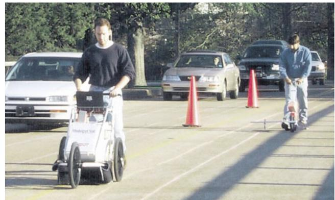
*Figure 2. The HollowDeck, in action, performs the same regardless of traffic conditions. In this particular configuration, a second operator lays down chalk lines to ensure consistent, accurate coverage of the deck.*
