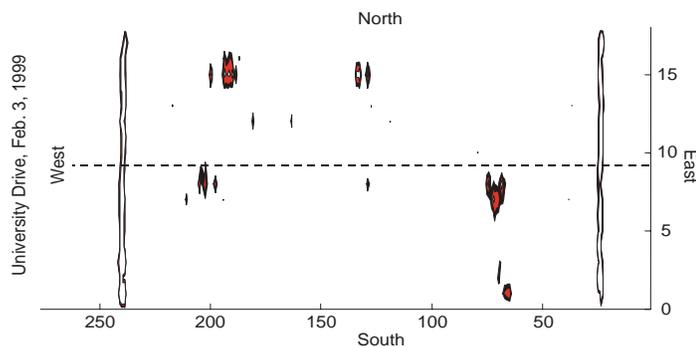
*Figure 3. Data collected from the University Drive Bridge over Highway 12, Starkville, MS. The dark bands on either end represent the expansion joints of the bridge. The colored areas represent areas detected by the HollowDeck, the block overlays are the results from “Expert” soundings.*
