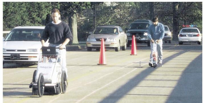
*Figure 2. The HollowDeck, in action, performs the same regardless of traffic conditions. In this particular configuration, a second operator lays down chalk lines to ensure consistent, accurate coverage of the deck.*
