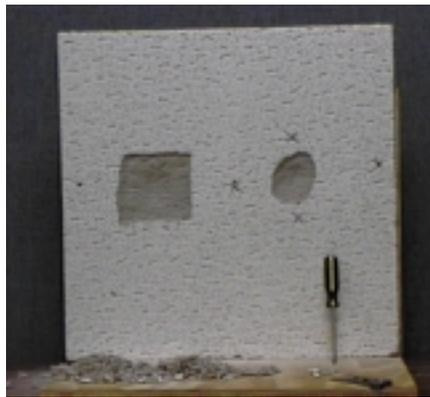
Figure 1 (above) Acoustical tile with gouged areas. Figure 2 (below) Grid lines, or pattern, projected onto left gouge of Figure 1.
